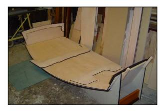
Before all that it is imperative that you make sure that the former assembly is going to give you a hull that is the right size and shape. To do that many hours of studying the measurement form and the drawings are required. I drew the bottom datum line onto the formers and marked off all the measuring points on the line, then checked that the drop to the underside of the curved hull bottom former was correct. It was. Then I made
