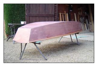
After any corrections and holes are filled, the next bit is to start the painting processes. There is a lot of this! I had glued the boat together with West System epoxy, which you can use as a clear two part liquid for close joints and then add filler powder to it to make up a paste of any consistency
